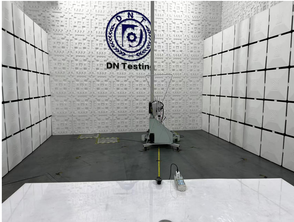
Radiated Emission Test View|(30M-1G)
