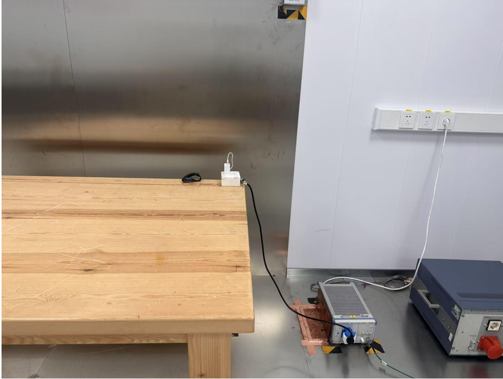
Radiated Emission Test View(9K-30MHz)
