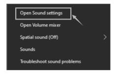
3. Select the "Sound Control Panel", go to the "Sound" settings, and set "TAKSTAR BN30B" as the default device for both "Playback" and "Recording" tabs. When speaking into the mic, the volume indicator icon will turn green and fluctuate.
