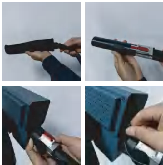
Figure 24. Schematic diagram of the connection between the emitter and the optical cable
