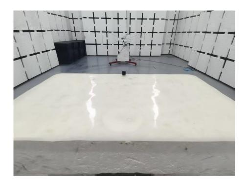
**Set-up for Radiated Spurious Emission, Above 1GHz**
