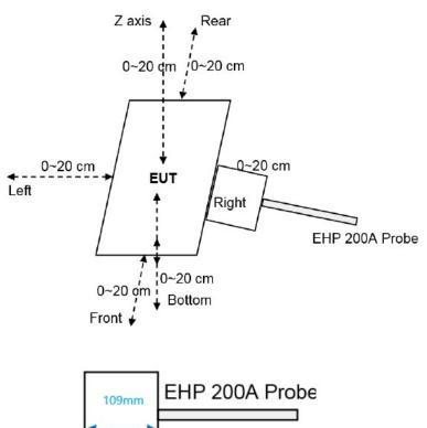
Notes: The EHP 200A Probe has a diameter of 10.9cm and a radius of 5.45cm
