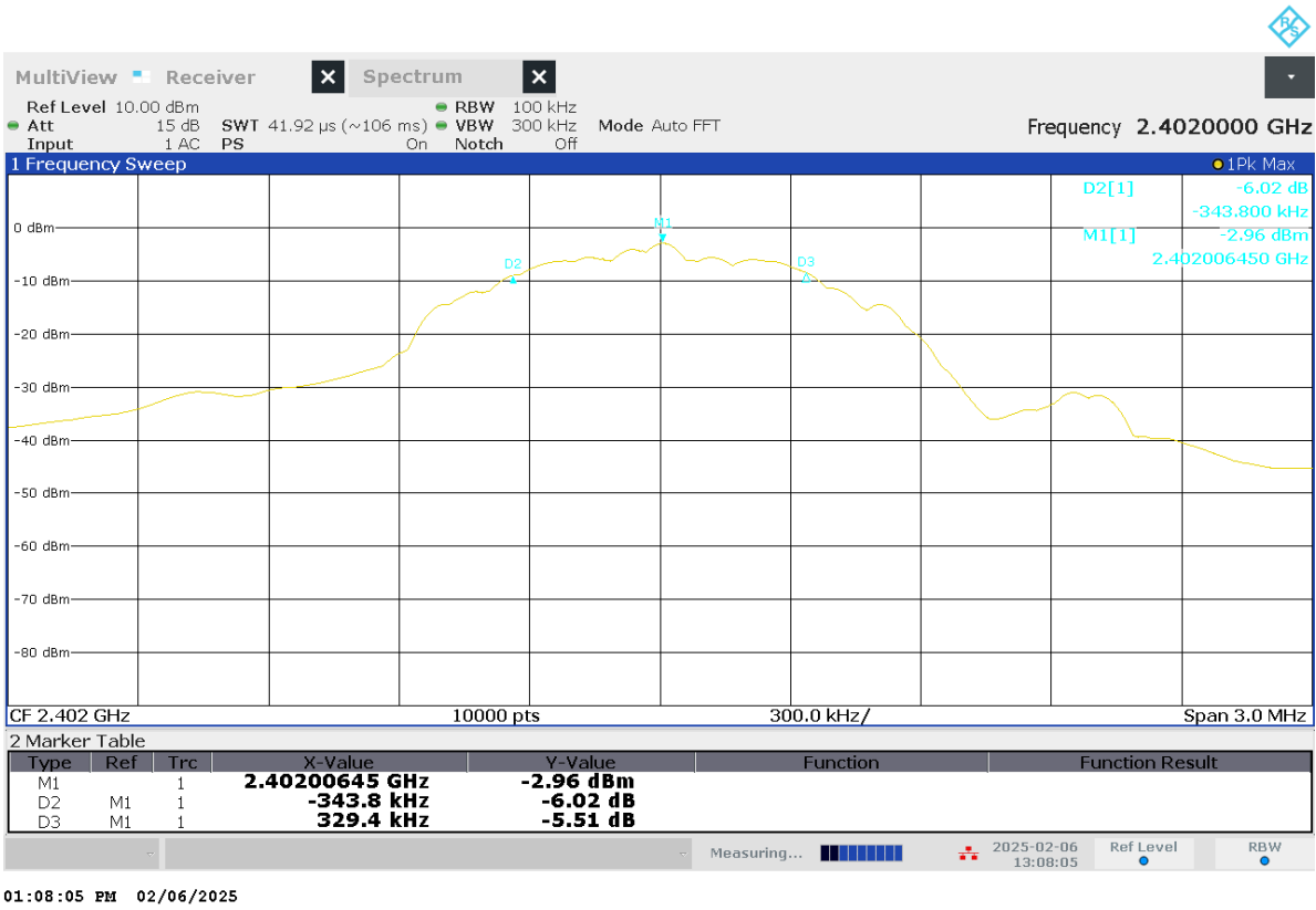
Figure 25 Bandwidth at 6dB Point. Operation on channel 2402MHz
