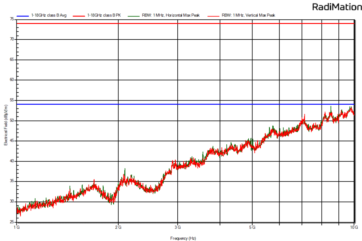
Figure 14 Electric field emissions Plot, 1GHz to 10GHz, Operation on 2402MHz - Peak detector scan – Puck Antenna
