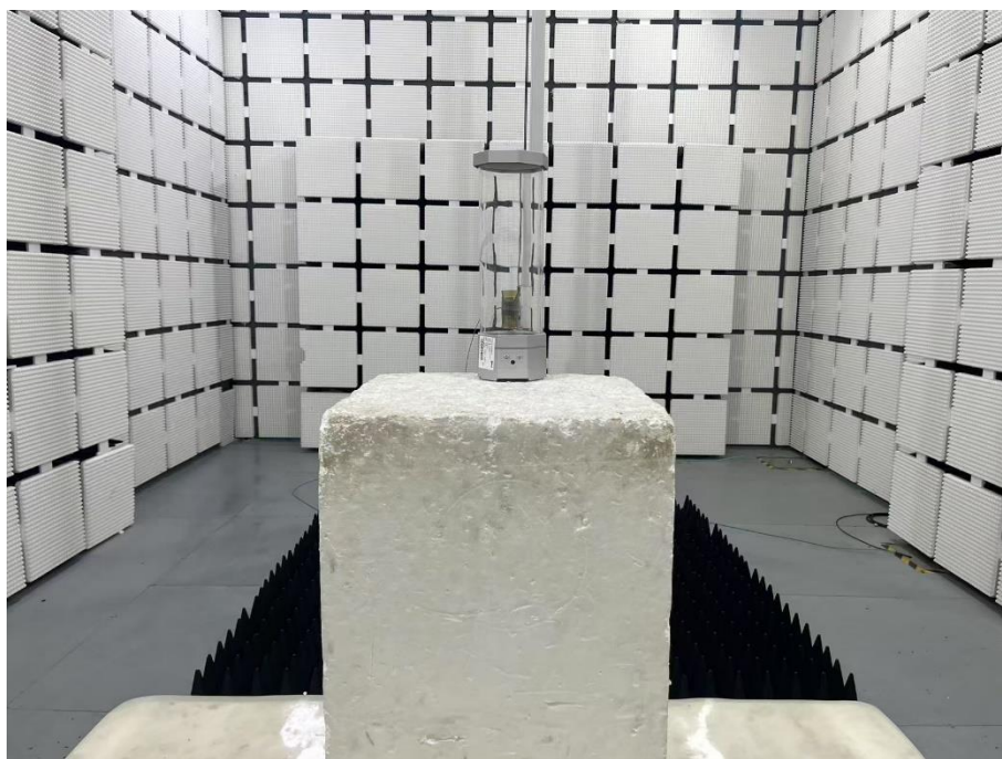
Set-up for Radiated Spurious Emission, Above 1GHz
