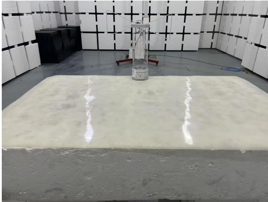
Set-up for Radiated Spurious Emission, Above 1GHz
