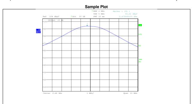
Offset applied accounts for antenna and cable losses and preamplifier gain.
