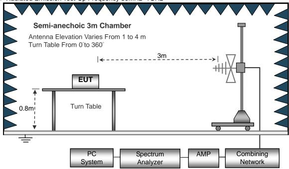
(C) Radiated Emission Test-Up Frequency Above 1GHz
