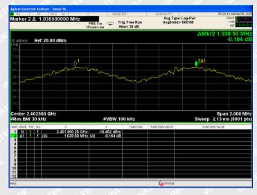
**GFSK\_Channel Separation\_Middle Channel**
