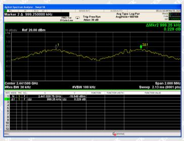
**GFSK\_Channel Separation\_High Channel**
