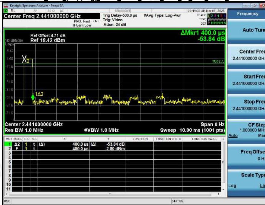
Dwell Time (Hopping) NVNT ANT1 1-DH1 2441 00 Accumulated
