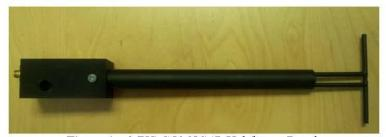
Figure 1 – MVG COMOSAR Validation Dipole
