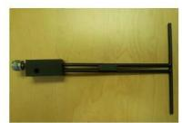
Figure 1 – MVG COMOSAR Validation Dipole
