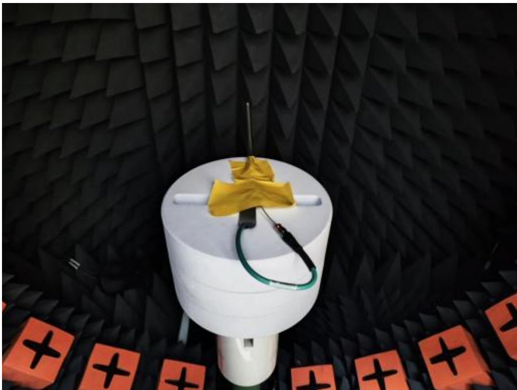
Product darkroom test environment diagram
