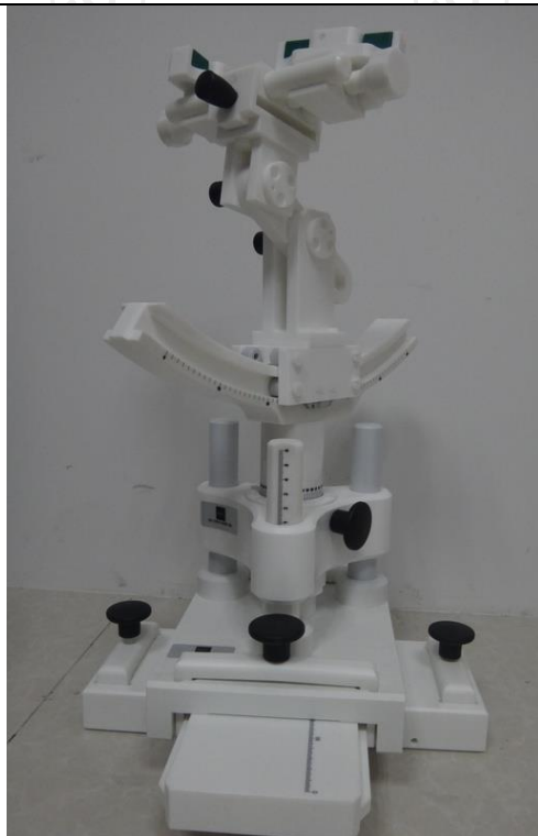
COMOSAR Mobile phone positioning system
