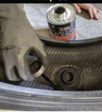
Apply bead sealer to the outer edge / perimeter of the patch.
