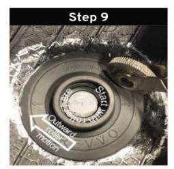
Apply Dock onto designated area with firm pressure, keeping arrows along the tire centerline. Use roller tool to apply even adhesion, starting from the center of the Dock and then moving to the outside in an outward fashion. Allow 1-2 minutes for Dock to bond.
