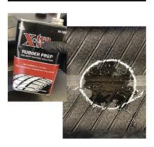
Pour enough rubber prep/pre-buff solution to cover designated installation area. Allow 30 seconds for solution to flash off.
