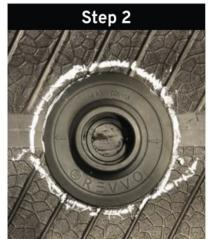
Outline dock with tire chalk to define area that will be prepped for proper Dock installation. Cover at least the circular area will the Dock will be installed. Area does not have to be a circle but must enclose the Dock's installation area.
