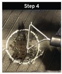
Use tire scraper tool to make 10-15 passes using firm force. This is to remove any excess chemicals to ensure surface is prepped.
