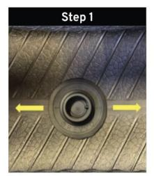
Outline Dock to ensure there are no defects. Align arrows and notch on dock with centerline on tire.
