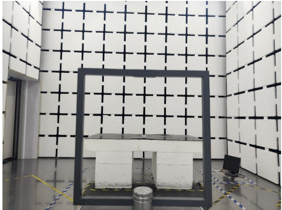
Radiation Emission Test Setup (Below 30MHz)
