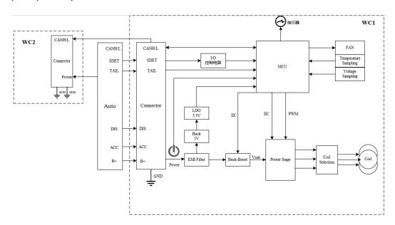
12V power supply. The 12V power supply is divided into two paths through EMI filter circuit. One path is converted into 3.3V to supply power to MCU through BUCK IC→LDO, and the other path is supplied with alternating current to the coil through Buck-Boost → Power Stage → Coil Selection, so that the coil generates electromagnetic field. When the coil of the mobile phone is put in, the energy can be transmitted to the mobile phone.
