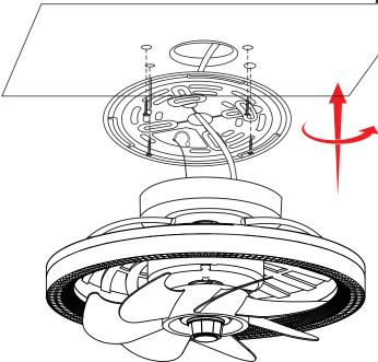
Install Step 1.Punch holes according to base hole position.
