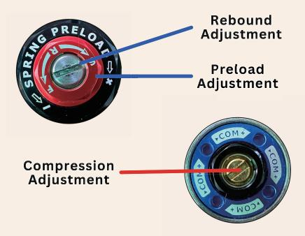
The AERO features a bidirectional dampening suspension on each side with rebound and dampening adjustment. The bidirectional dampening feature allows the same coil to fit more weight classes of riders.
