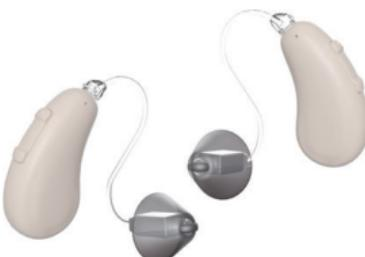
Open the charging case and take out the hearing aid. It will automatically power on and enter the pairing mode after 10 seconds. You will hear the voice prompt "Enter pairing mode", and at the same time, the white light will flash, putting it into the pairing state.
