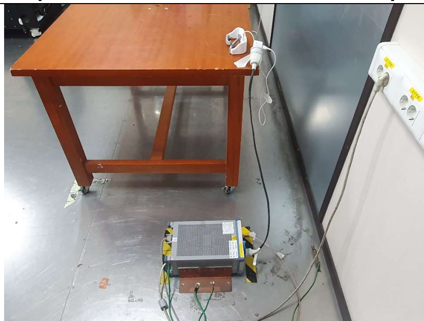
[Rear view of Continuous Conducted Emission at main]
