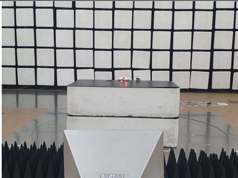
[Rear view of Radiated Emission (Above 1GHz)]
