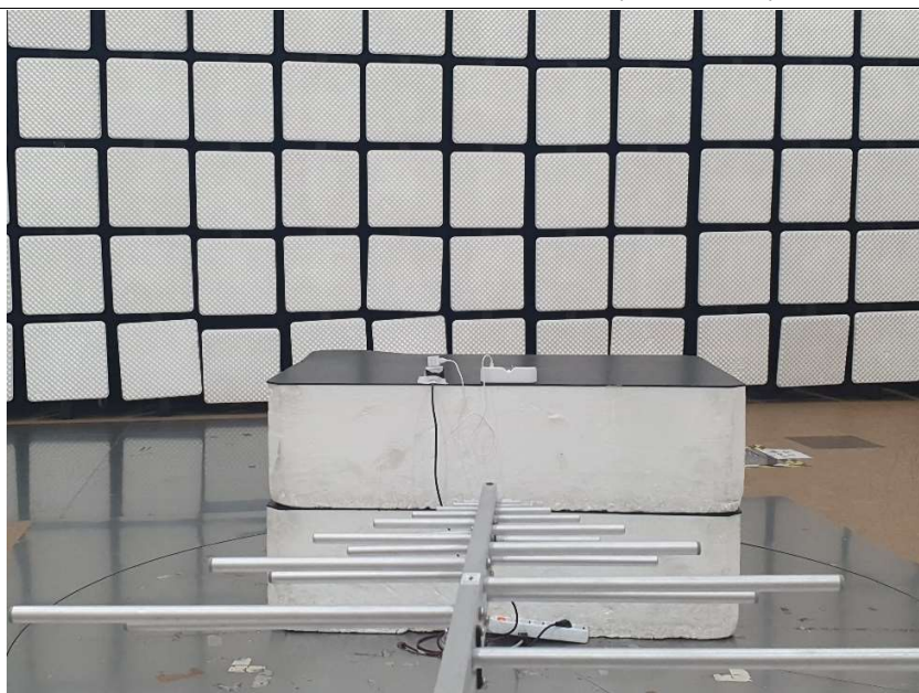
[Rear view of Radiated Emission (Below 1GHz)]
