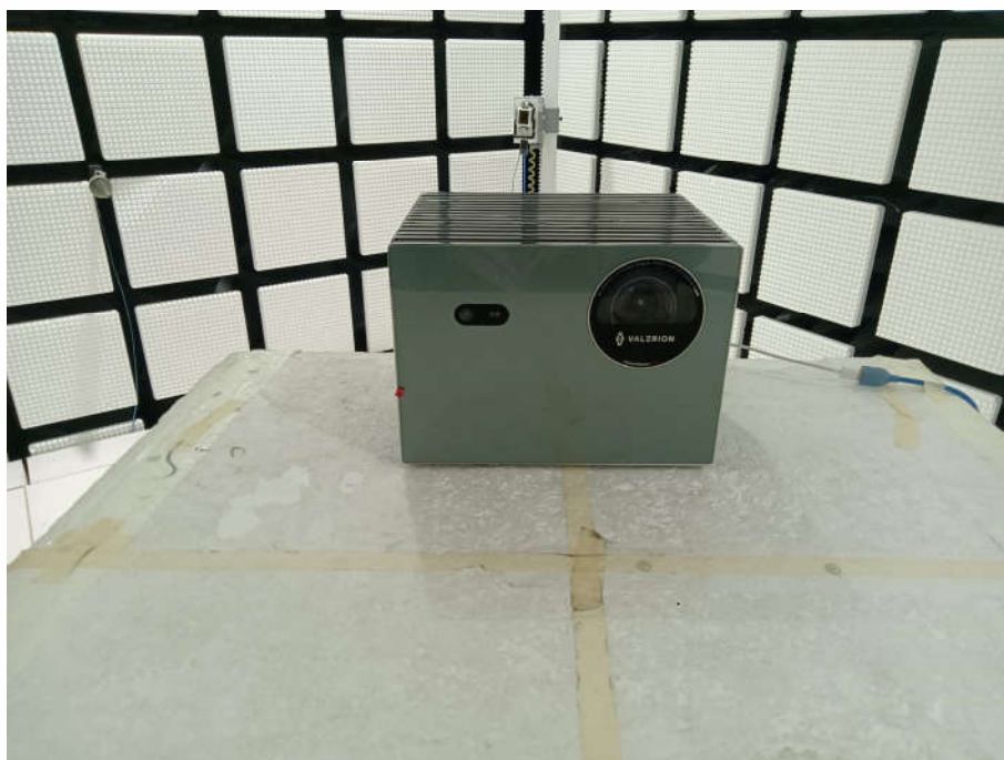
Radiated spurious emission Test Setup-2(Above 1GHz)
