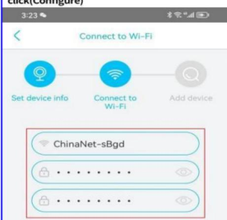
The device does not currently support 5GHz WiFi bands. Please make sure your phone is connected to a 2.4GHz WiFi band, then raise the volume of your phone and keep it a few inches away from the device while it connects
