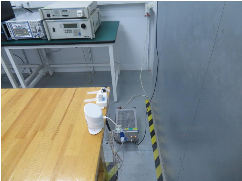
Description: Back View of Conducted Emission Test Setup for Power Port (For Radar)
