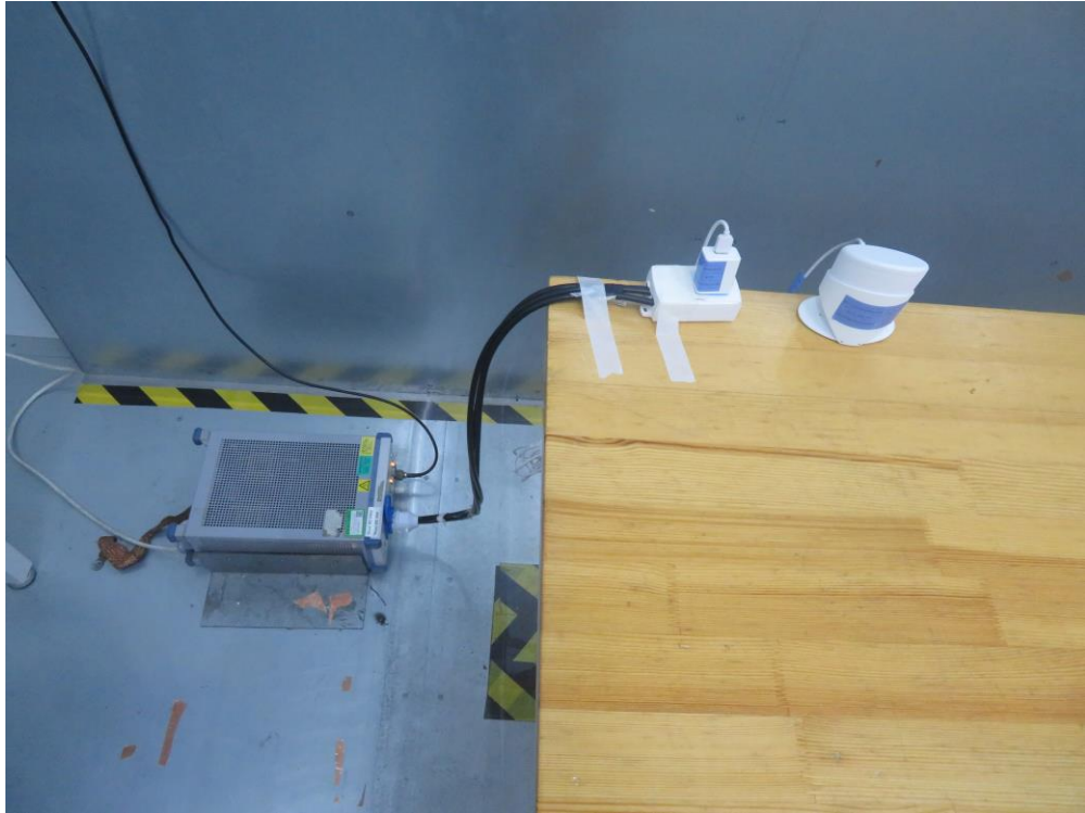
Description: Back View of Conducted Emission Test Setup for Power Port (For Radar)
