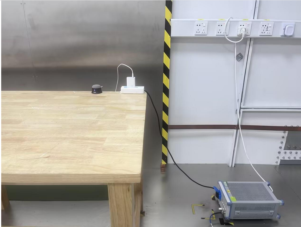
AC Power Line Conducted Emission
