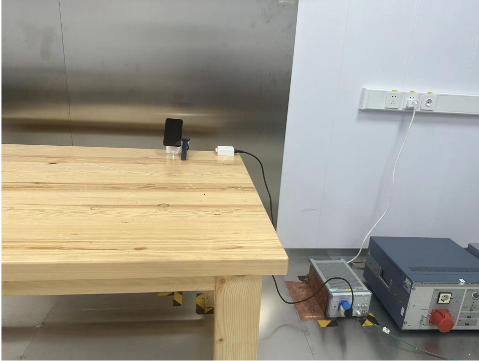
Radiated Emission Test View|(9K- 30MHz)
