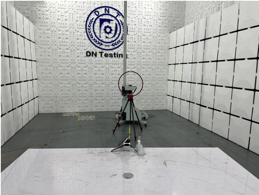
Radiated Emission Test View|(9K- 30MHz)
