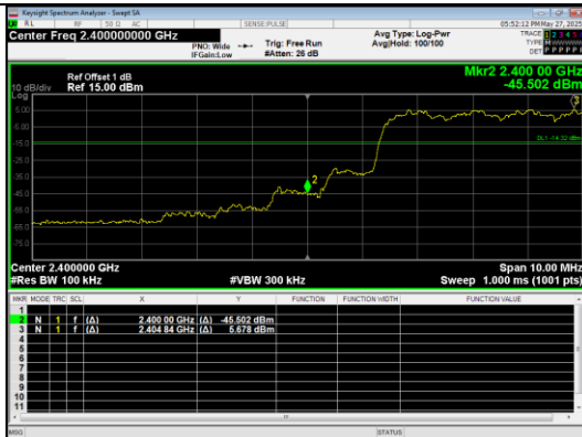
Out Of Band Emission(Left) 8DPSK_3-DH5_Channel Hopping
