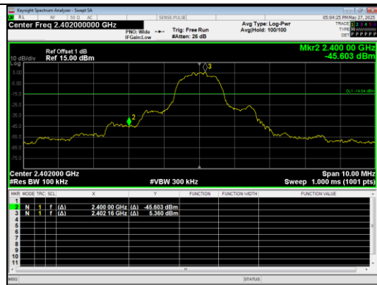
Out Of Band Emission 8DPSK_3-DH5_Channel 0
