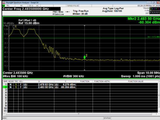
Out Of Band Emission(Right) GFSK_DH5_Channel Hopping
