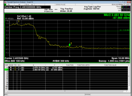
Out Of Band Emission(Right) \pi/4 DQPSK_2-DH5_Channel Hopping
