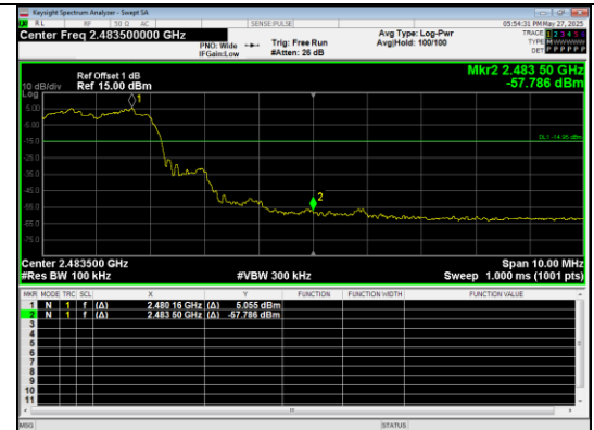
Out Of Band Emission(Right) 8DPSK_3-DH5_Channel Hopping
