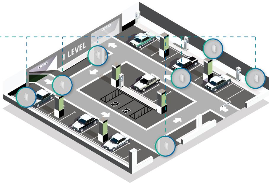
The Optergy Air BW-THCO-M sensor pairs with the Optergy Air Transceiver (BG-1000-M). Up to seven (7) Optergy Air BW-THCO-M sensors can be connected to one Optergy Air Transceiver (BG-1000-M).
