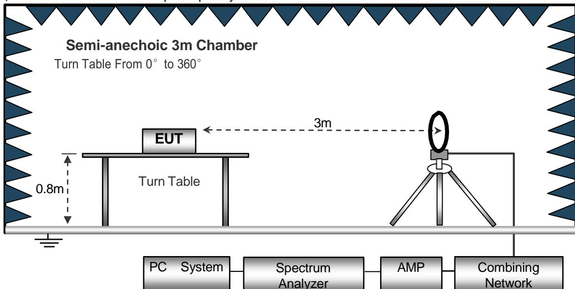
( B ) Radiated Emission Test-Up Frequency 30MHz~1GHz
