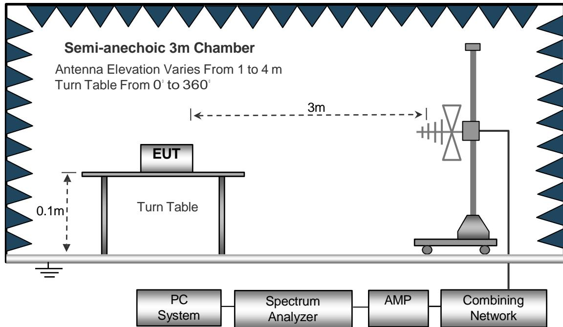
( C ) Radiated Emission Test-Up Frequency Above 1GHz
