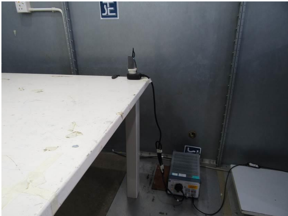
Measurement of Conducted Emission Test Set Up
