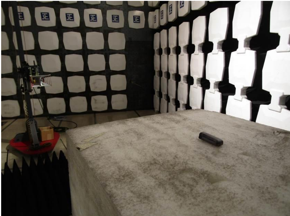
Measurement of Conducted Emission Test Set Up
