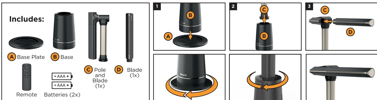
1. Use assembly stickers to align the **Base** onto the **Base Plate**. Rotate the base clockwise until it clicks into place.
