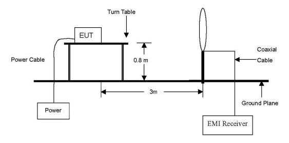
The diagram below shows the test setup that is utilized to make the measurements for emission from 30  $\,\mathrm{M}\!\mathrm{L}$  to 1  $\,\mathrm{GL}$  emissions.
