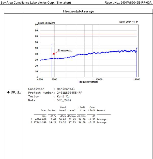
Note: Spectrum analyzer setting: RBW=1 MHz, VBW=5 kHz
