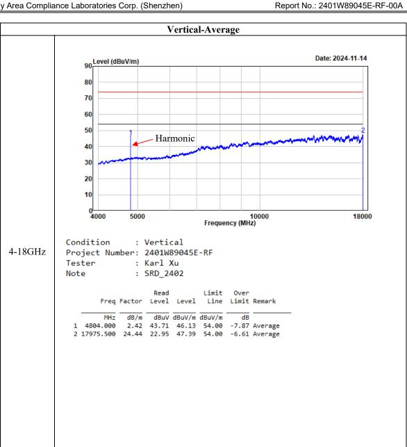
Note: Spectrum analyzer setting: RBW=1 MHz, VBW=5 kHz
