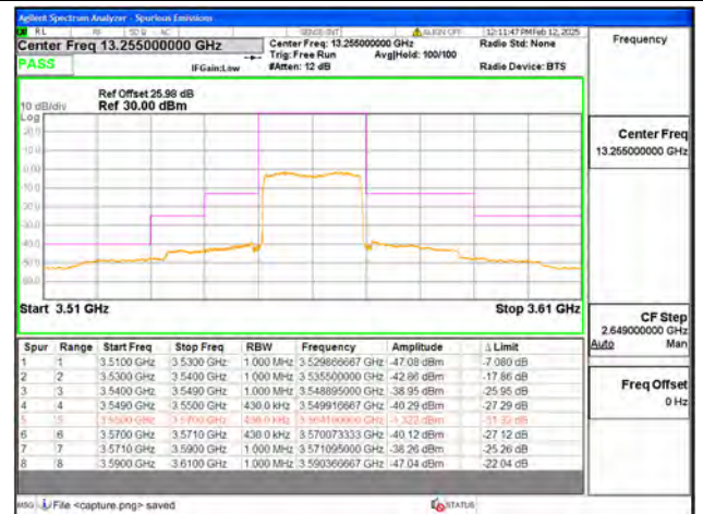
B48 / 20MHz / Low CH / QPSK / FULL RB
