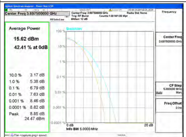
B48 / 5MHz / High CH / 256QAM
