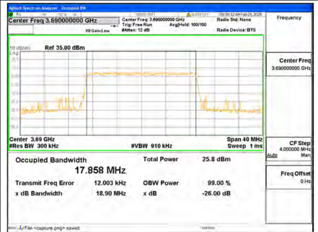
B48 / 20MHz / 16QAM/ High CH
