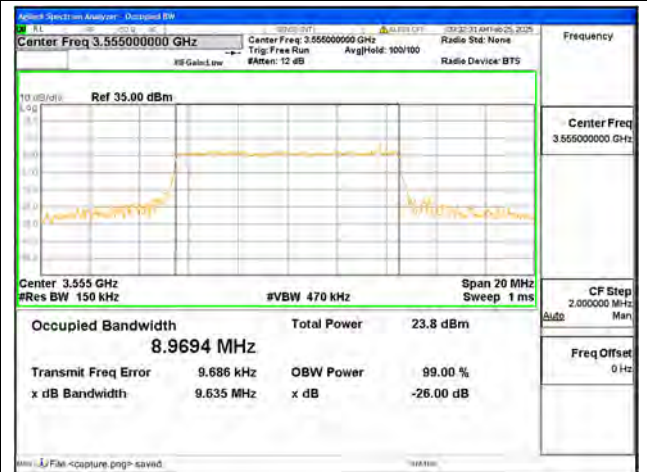
B48 / 10MHz / 256QAM/ Low CH
