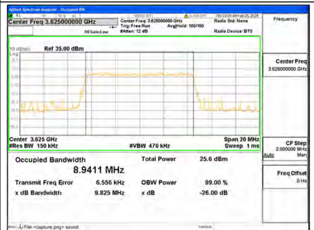
B48 / 10MHz / 16QAM/ Mid CH
