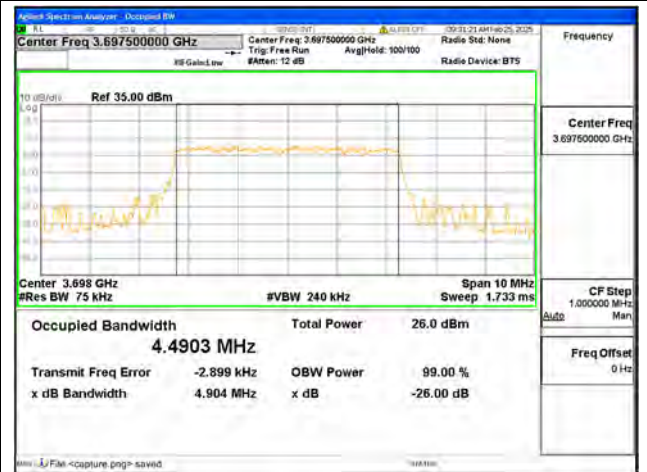
B48 / 5MHz / 16QAM/ High CH
