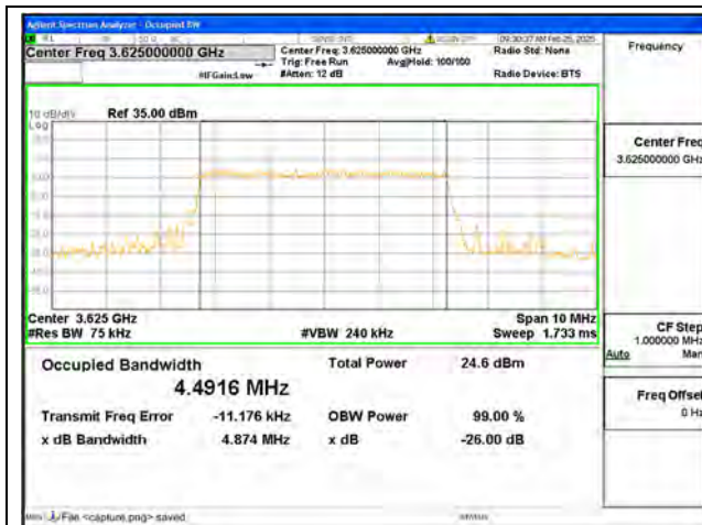
B48 / 5MHz / 64QAM/ Mid CH
