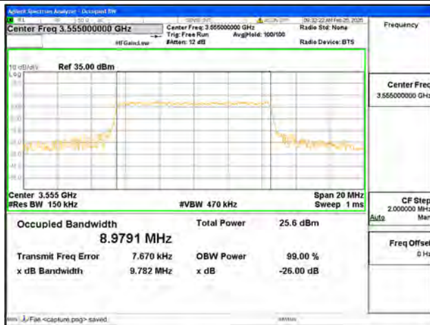
B48 / 10MHz / 64QAM/ Low CH
