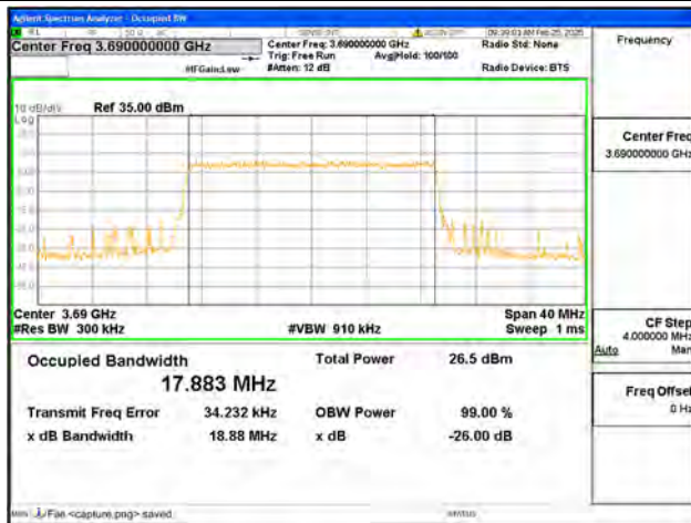
B48 / 20MHz / QPSK/ High CH
