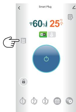
If there is no installed sensor be detected, the icon would be hidden.
