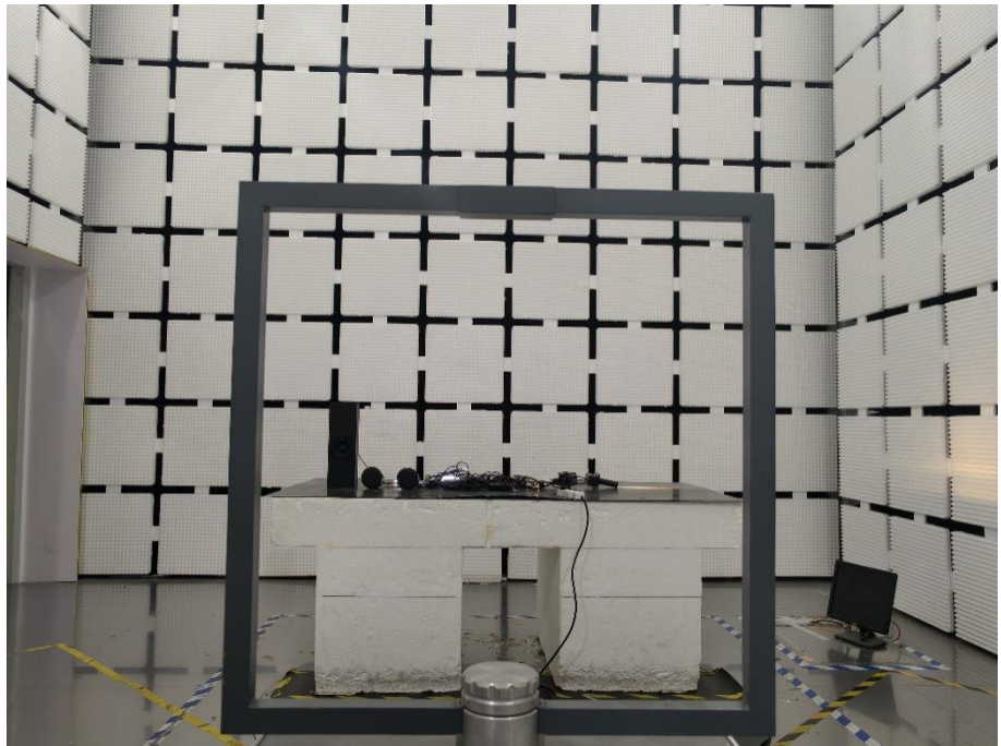
Radiation Emission Test Setup (Below 30MHz)
