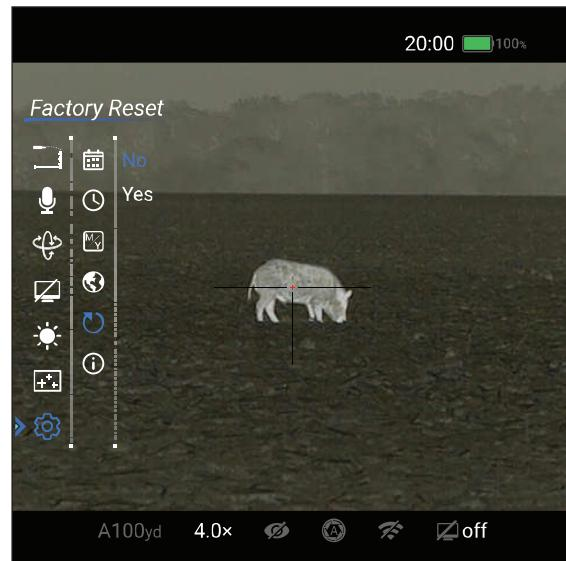
5. Short press the **Up ▲** or **Down ▼ Button** to select **No** and short press the **Menu M Button** to confirm cancellation of the factory reset and return to the submenu.
