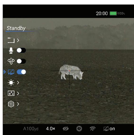
3. Short press the **Menu M Button** to toggle auto standby on / off When turned on, the RICO 2 will automatically enter standby after about 5 seconds of inactivity.
