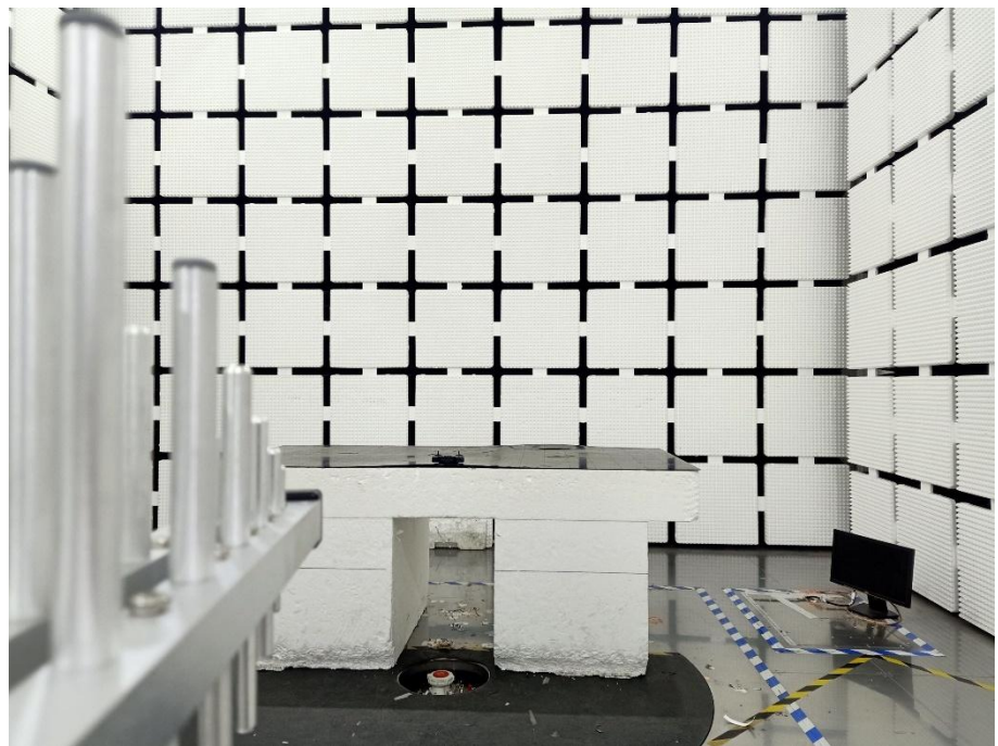
Radiation Emission Test Setup (30MHz to 1GHz)
