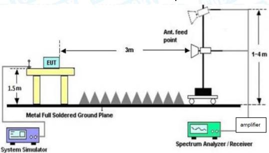
**Above 1GHz Test Setup**
