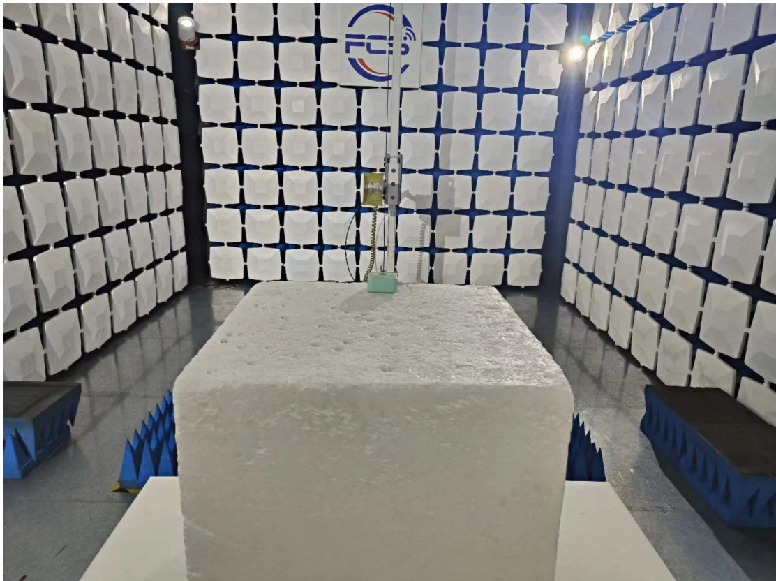
Above 1GHz for radiated emission test setup
