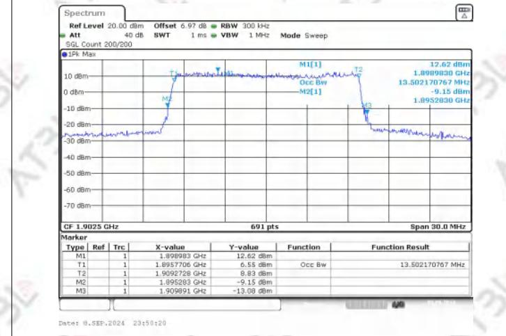
Band2 QAM16 BW=15MHz Channel=19125 RB Size=75 Position=#0 NVNT
