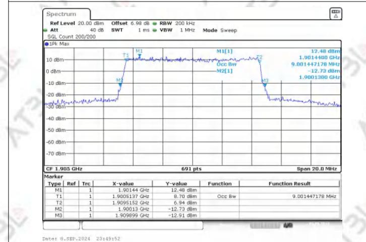
Band2 QAM16 BW=10MHz Channel=19150 RB Size=50 Position=#0 NVNT
