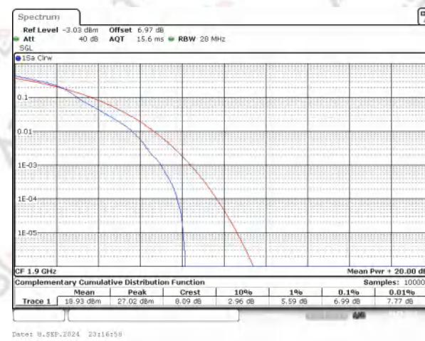
Band2 QAM16 BW=20MHz Channel=19100 RB Size=1 Position=#0 NVNT
