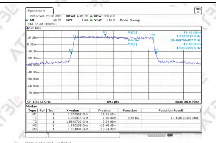
Band2 QAM16 BW=15MHz Channel=18675 RB Size=75 Position=#0 NVNT
