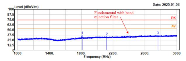
Condition: PK RBW:1MHz VBW:3MHz SWT:auto Limit Polarity Freq Reading Factor Result Margin Remark MHz dBuV dB/m dBuV/m dBuV/m dΒ 1811.80 50.92 -13.47 37.45 74.00 36.55 horizontal Peak 34.53 74.00 39.47 horizontal Peak 2118.80 46.26 -11.73 2764.20 46.68 -9.29 37.39 74.00 36.61 horizontal Peak
