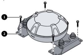
Method 2: Use the 3M stickers 2 to fix the GNSS receiver bracket 1.
