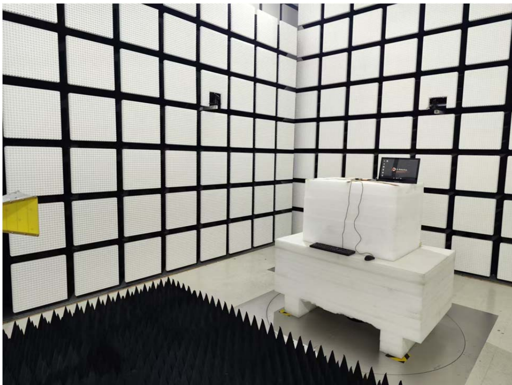
Radiated Emission Above 1-18GHz View RDK X5 4G
