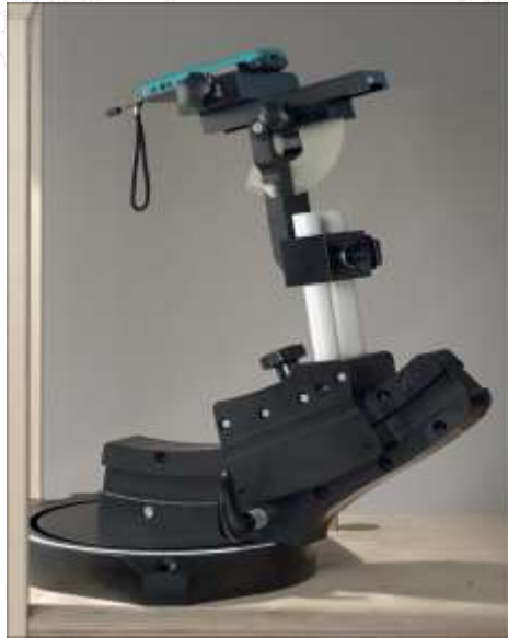
F-2. Device Holder for Transmitters
