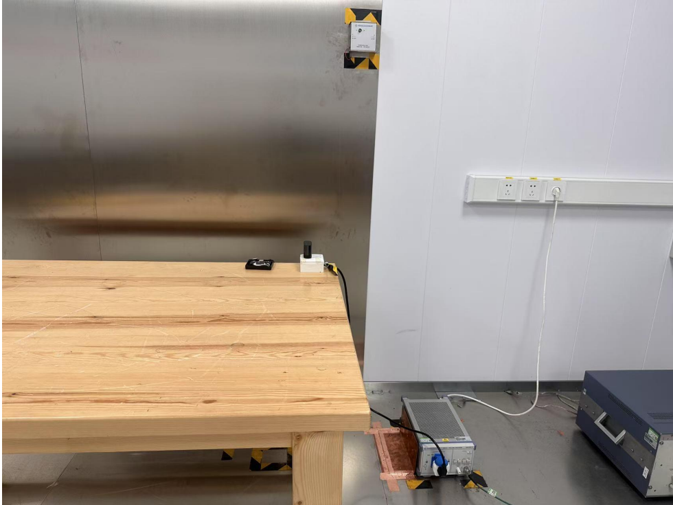
Radiated Emission Test View|(Below 1G)
