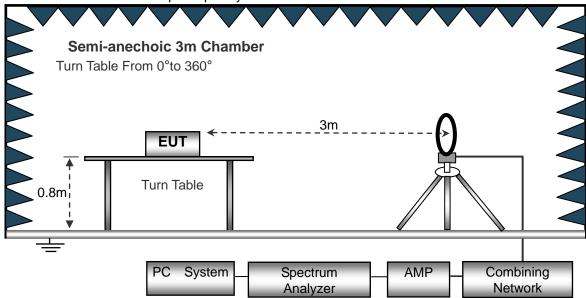
(B) Radiated Emission Test-Up Frequency 30MHz~1GHz
