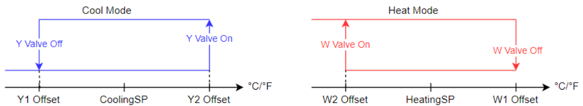
FIGURE 19: TWO PIPE COOLING AND HEATING MODE
