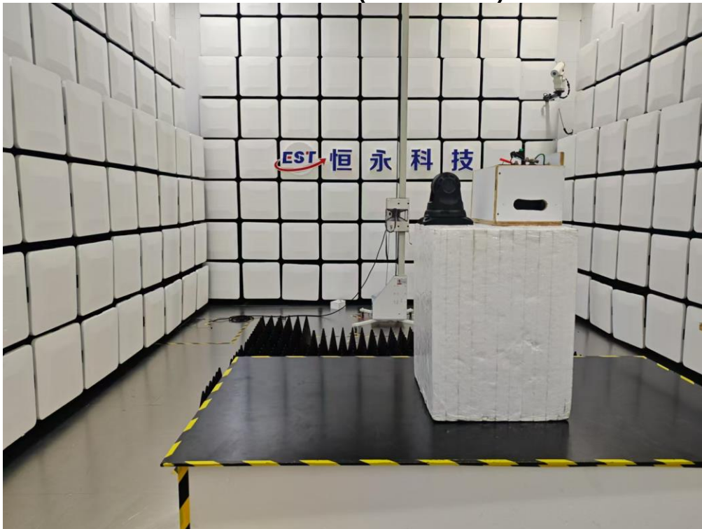
Radiated Test (Above 1GHz)
