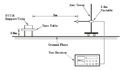
The radiated emissions were performed in the 3 meters distance, using the setup accordance with the ANSI C63.10-2020. The specification used was the FCC 15.209 and FCC Part 15.235(a) & 15.235 (b) limits.
